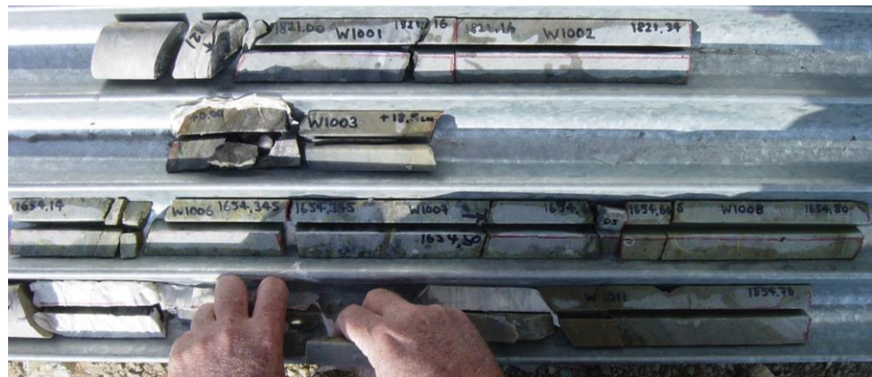
Figure 24: Sawn core from borehole WR1 (Basal Reef) deflections 0 and 2 showing removal of masking tape (used by AAC to preserve friable portions of the core) prior to sawing
