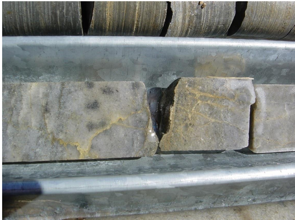
Figure 22: Core recovery: Complete loss of bottom contact in borehole HB1
